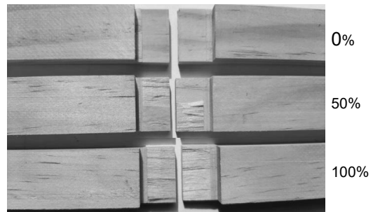
Figure 3. Wood failure percentage examples with wood failure 0%, 50% and 100%.
