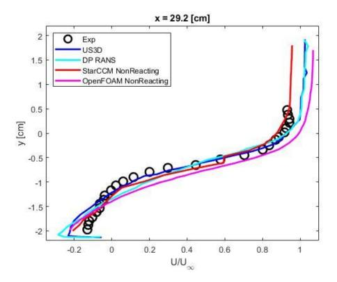
Figure 49: 29.2 cm X-Component Data for Non-Reacting RANS
