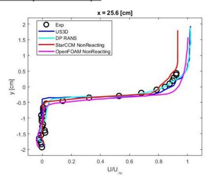
Figure 45: 25.6 cm X-Component Data for Non-Reacting RANS
