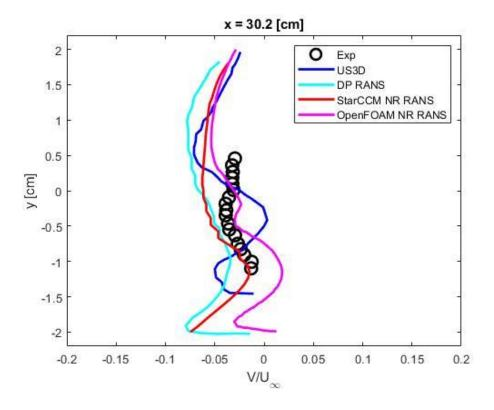
Figure 57: 30.2 cm Y-Component Data for Non-Reacting RANS
