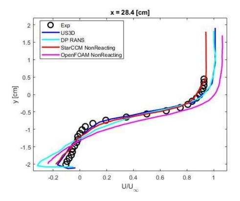
Figure 48: 28.4 cm X-Component Data for Non-Reacting RANS
