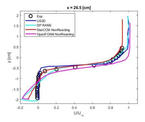
Figure 46: 26.5 cm X-Component Data for Non-Reacting RANS
