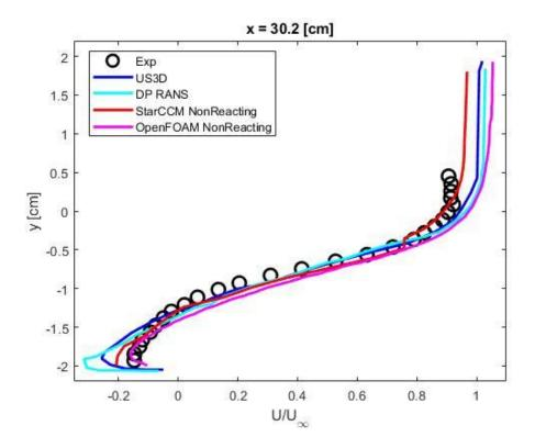
Figure 50: 30.2 cm X-Component Data for Non-Reacting RANS
