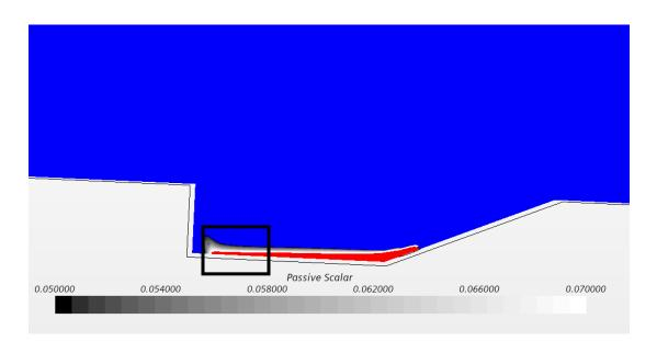
Figure 94: StarCCM Combustion Location using RANS
