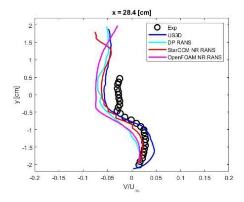
Figure 55: 28.4 cm Y-Component Data for Non-Reacting RANS
