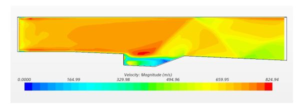
Figure 17: Velocity Scene of Simple Flame Holder Cavity
