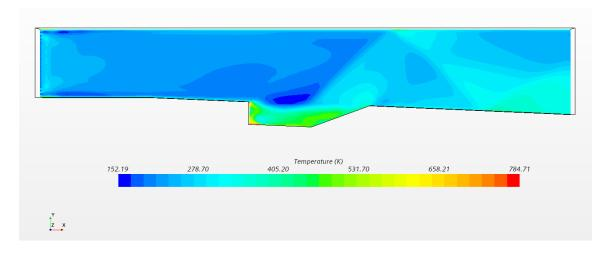
Figure 18: Temperature Scene of Simple Flame Holder Cavity
