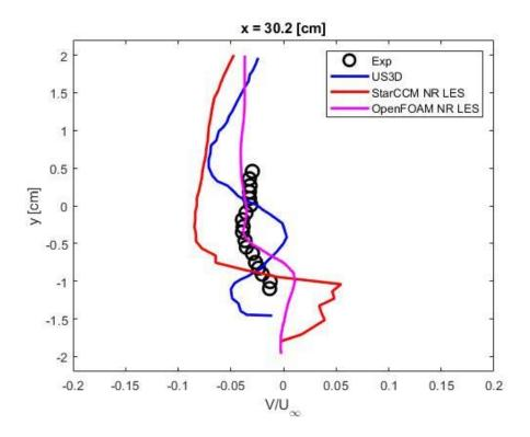
Figure 75: 30.2 cm Y-Component Data for Non-Reacting LES
