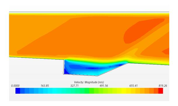
Figure 25: RANS No Injector Velocity Scalar Scene
