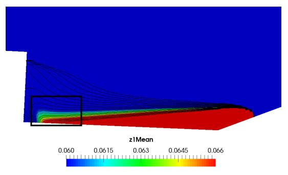
Figure 95: OpenFOAM Combustion Location using RANS
