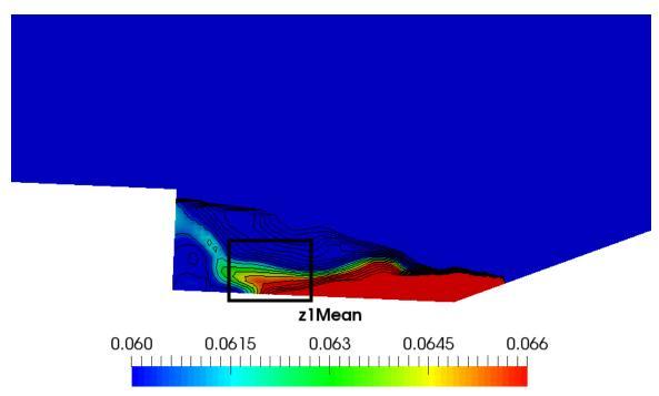
Figure 97: OpenFOAM Combustion Location using LES
