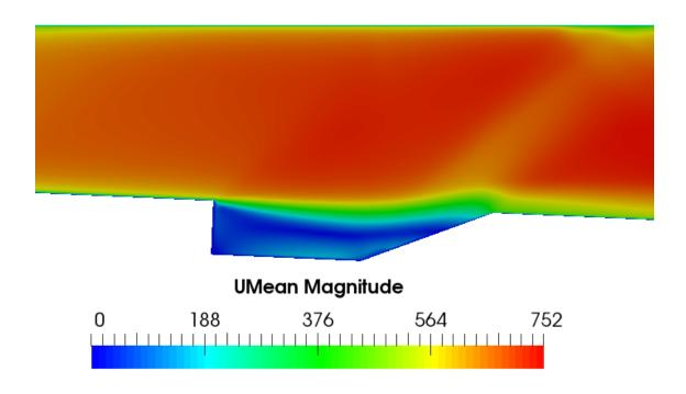
Figure 38: Non-Reacting RANS OpenFOAM Velocity Scene
