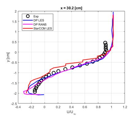
Figure 36: 30.2 cm Data for LES with No Injection
