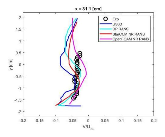
Figure 58: 31.1 cm Y-Component Data for Non-Reacting RANS
