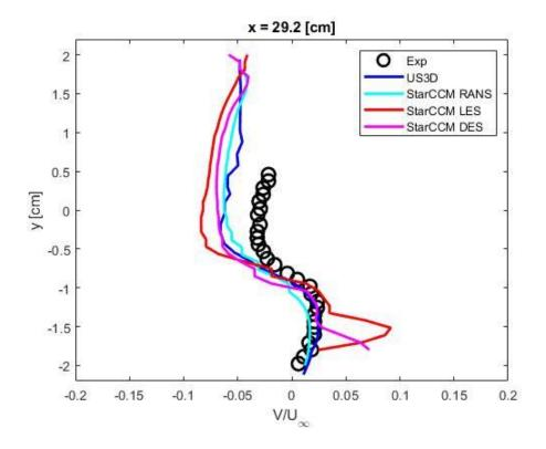
Figure 91: 29.2 cm Y-Component Data for Non-Reacting DES
