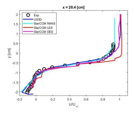
Figure 83: 28.4 cm X-Component Data for Non-Reacting DES
