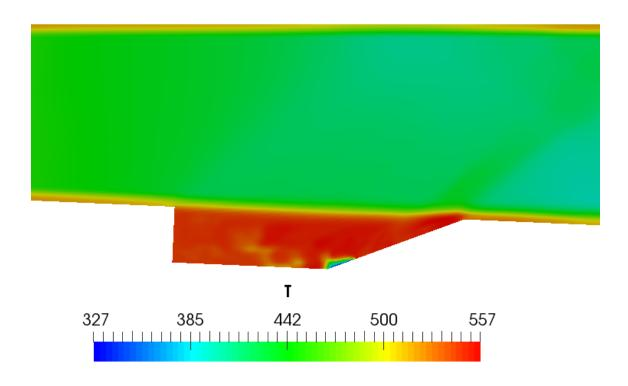
Figure 65: Non-Reacting LES OpenFOAM Temperature Scene
