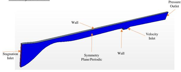
Figure 15: Model with Boundary Conditions
