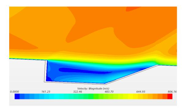
Figure 37: Non-Reacting RANS StarCCM Velocity Scene
