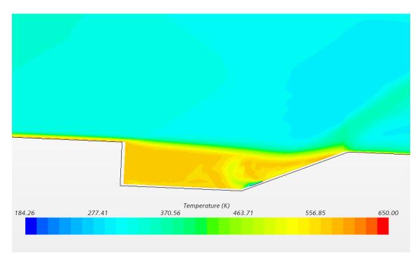
Figure 64: Non-Reacting LES StarCCM Temperature Scene
