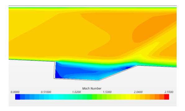
Figure 27: RANS No Injector Mach Number Scalar Scene
