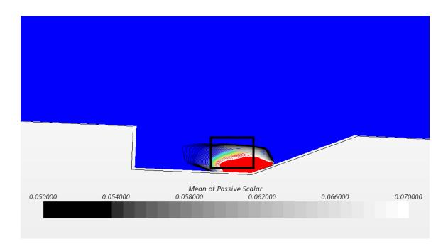
Figure 96: StarCCM Combustion Location using LES
