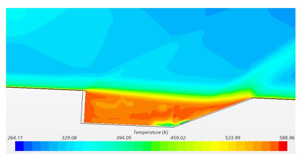
Figure 77: Non-Reacting DES StarCCM Temperature Scene
