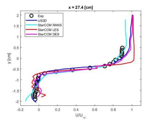
Figure 82: 27.4 cm X-Component Data for Non-Reacting DES
