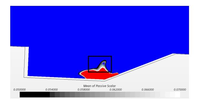
Figure 98: StarCCM Combustion Location using DES
