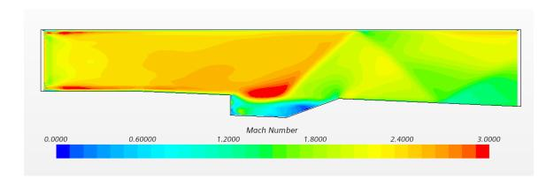
Figure 19: Mach Number Scene of Simple Flame Holder Cavity
