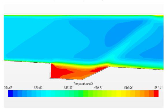
Figure 26: RANS No Injector Temperature Scalar Scene
