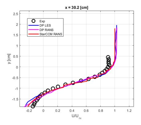
Figure 30: 30.2 cm Data for RANS with No Injection
