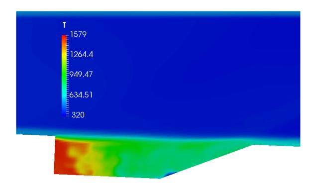
Figure 59: OpenFOAM Temperature Scene for 0.01 Second LES Case
