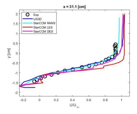
Figure 86: 31.1 cm X-Component Data for Non-Reacting DES
