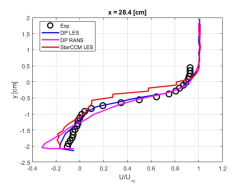
Figure 35: 28.4 cm Data for LES with No Injection
