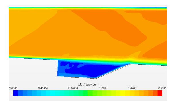
Figure 33: LES No Injector Mach Number Scalar Scene
