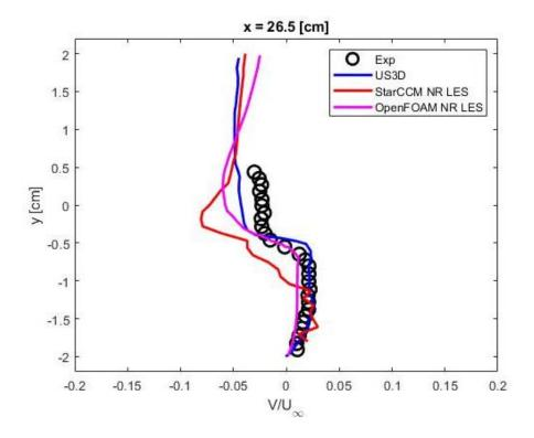
Figure 73:26.5 cm Y-Component Data for Non-Reacting LES
