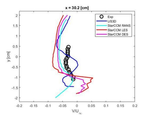
Figure 92: 30.2 cm Y-Component Data for Non-Reacting DES
