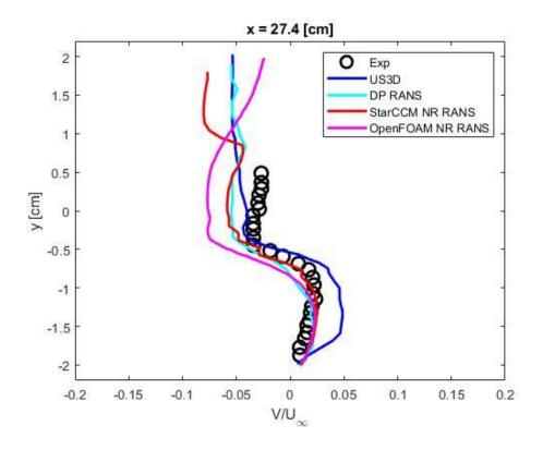
Figure 54: 27.4 cm Y-Component Data for Non-Reacting RANS
