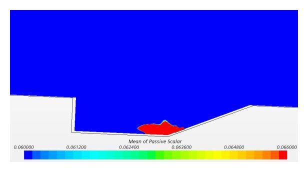
Figure 78: Non-Reacting DES StarCCM Mean Passive Scalar Scene
