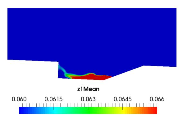
Figure 67: Non-Reacting LES OpenFOAM Mean Passive Scalar Scene
