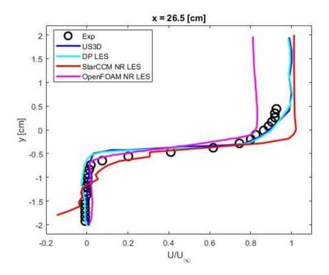
Figure 70: 26.5 cm X-Component Data for Non-Reacting LES
