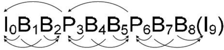
Figure 4.7: Typical Structure of a Group-of-Pictures (GoP) in a MPEG Video Stream. Reproduced from [3].
