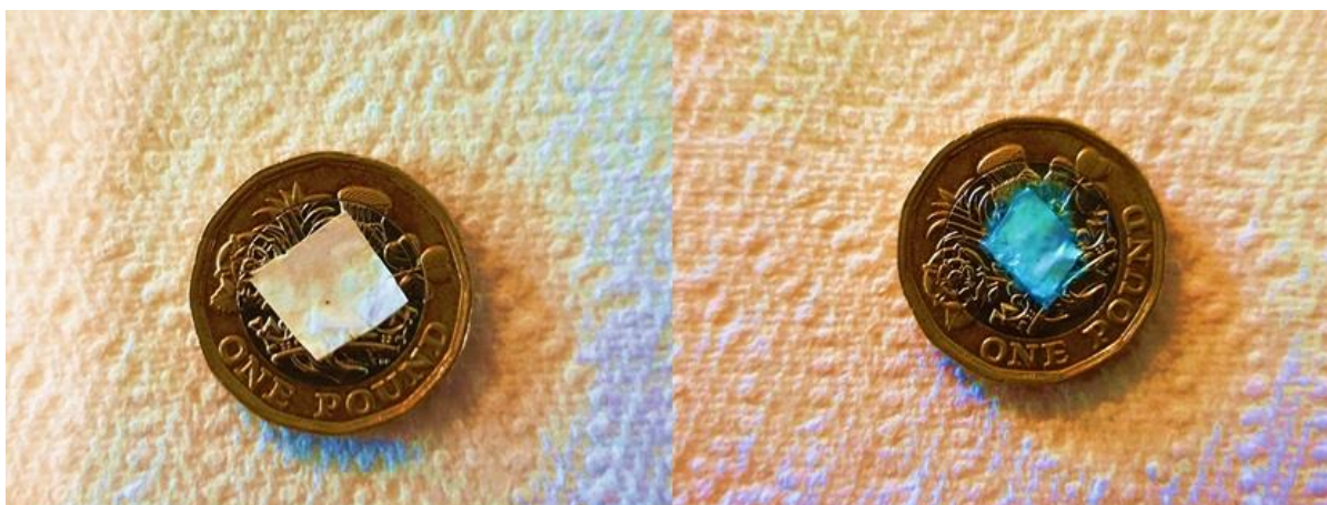
Figure 3.5 The contrast between hue of chitosan-coated porous PLLA nanofibres without and with adsorption of Cu (II) ions.
