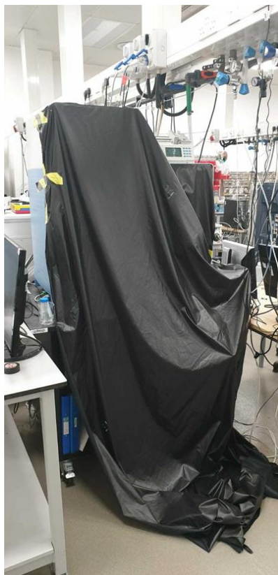
SI Figure 1: Black out curtain around the Q-exactive UHMR UHMR mass spectrometer to block out any laboratory light.
