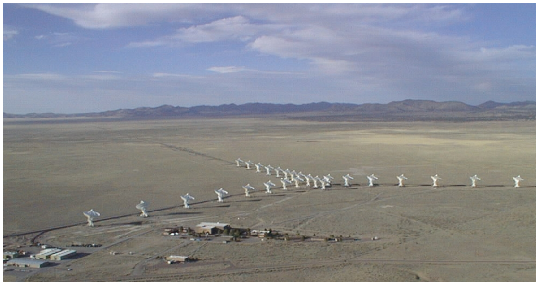
Figure 3.1: Antennas in the JVLAs array are moved every few months to observe with different resolutions. This is an image of the JVLAs in C configuration ( b_{max} = 3.4 km). Photo credit: NRAO, NSF.
