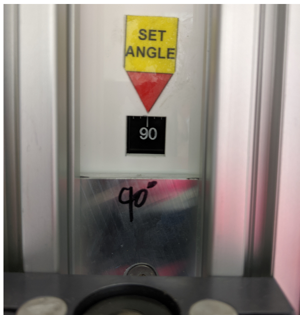
Figure 5.6: Close up image of the angle selection wheel and window.
