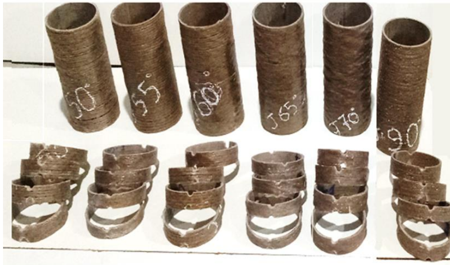
Fig. 3 – Specimens for stiffness and hoop tension
