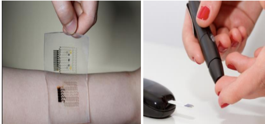
Figure 1.1 Images of a wearable glucose sensing device monitoring blood glucose via sweat (Left) and the traditional blood glucose monitoring technique of a finger stick blood test (Right).
