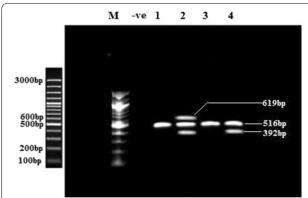
**Fig. 1** Agarose gel electrophoresis of multiplex PCR for ESBLs genes detection including  $bla_{\rm OXA1}$ ,  $bla_{\rm TEM}$ ,  $bla_{\rm SHV}$ . M: 100 bp DNA marker (Thermo-scientific), -ve: blank controls, 1:  $bla_{\rm OXA1}$  (619 bp), 2: multiple genes including  $bla_{\rm OXA1}$  (619 bp),  $bla_{\rm TEM}$  (516 bp), and  $bla_{\rm SHV}$  (392 bp), 3:  $bla_{\rm TEM}$  (516 bp), 4: multiple genes including  $bla_{\rm TEM}$  (516 bp), and  $bla_{\rm SHV}$  (392 bp)
