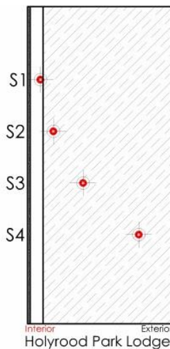
Figure 3 - Location of sensors for indoor conditions monitoring and in-wall monitoring (28)
