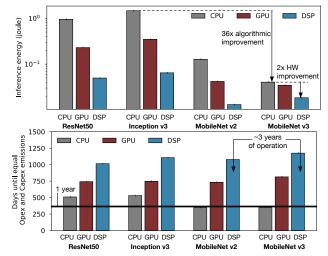
Fig. 3. Evaluating carbon footprint between manufacturing- and operationalrelated activities for Google Pixel 3 smartphone. Algorithmic AI and hardware advances dramatically shifted carbon emissions toward manufacturing overhead. The top shows the algorithm-level and hardware-level energy improvements for mobile AI inferences. The bottom chart shows how many days of image processing is necessary for operational output to equal integratedcircuit-manufacturing output.
