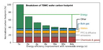
Fig. 5. Carbon-emissions breakdown for TSMC wafer manufacturing. Renewable energy provides up to a  $64 \times$  reduction in emissions from electricity, and overall emissions for wafers drops by  $2.7 \times$ . Although the reduction will reduce the carbon output of manufacturing, consideration of capex-related emissions for mobile and data-center hardware will remain important.
