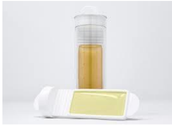
Image 4-1 Agar gel dip-slides for quantification of culturable coliforms and E. coli
