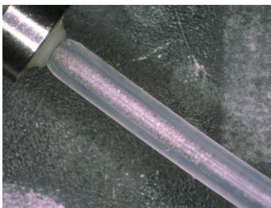
Figure D.4. Picture of the trickle-bed capillary reactor made of PTFE tube (ID: 1 mm) containing 7 mg of packed 1 wt% Au-Pd/TiO 2 catalyst with a particle size 90-125 μm.
