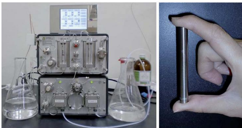
Figure 2.3. Picture of the XCube™ flow reactor (left) and the catalyst cartridge (right). Reprinted from Osako et al. , Continuous-flow hydrogenation of olefins and nitrobenzenes catalyzed by platinum nanoparticles dispersed in an amphiphilic polymer, RSC Advances, 2015, 5, 45760-45766, with permissions from the Royal Society of Chemistry.
