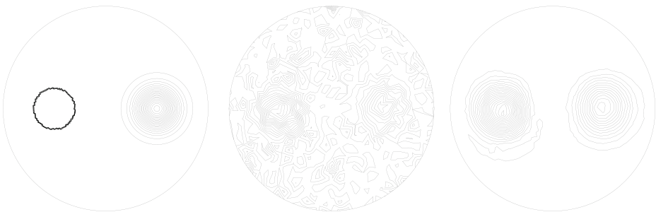
Fig. 2 From left to right: rough initial data on fine mesh u_0 + \tilde{u}_0 , unstabilized solution, stabilized solution ( n_{ele} = 80 , one turn)
