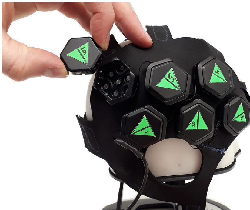
Figure 6.1: The wearable Gowerlabs LUMO device, used by Frijia et al. to study responses in the infant brain. Figure adapted from Frijia et al. (2021), licensed under CC BY 4.0 .
