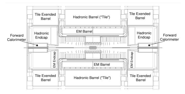
**Figure 3.5.:** Cross-sectional view of the calorimetry system in the ATLAS detector. This figure is from Ref. [27].
