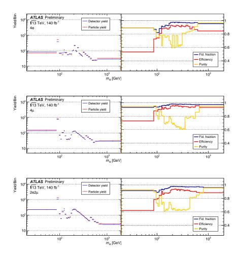
**Figure A.3.:** In the left-hand panels, the number of predicted events passing the reconstructionand fiducial- level selections are displayed as the detector yield and particle yield, respectively. The right-hand panel shows the efficiency, fiducial purity and fiducial fraction. All variables are plotted as a function of the  $m_{4\ell}$  bins, in the 4*e*, 4 $\mu$  and 2*e*2 $\mu$  flavour channels from top to bottom.
