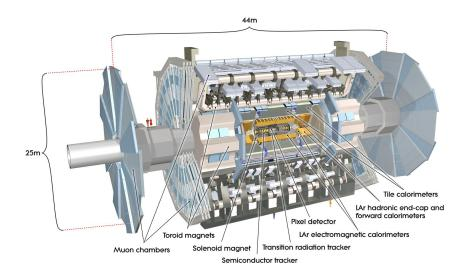
Figure 3.4.: The ATLAS detector and its sub-components. This figure is from Ref. [19].
