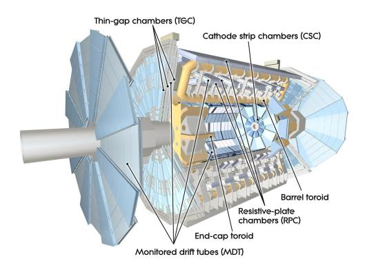
**Figure 3.6.:** A section view of the ATLAS Muon Spectrometer and its sub-components. This figure is from Ref. [34]
