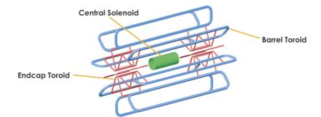
Figure 3.7.: Schematic representation of the ATLAS magnet system. This Figure is from Ref. [36].
