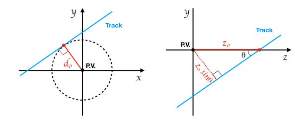
**Figure 3.8.:** Drawn in blue is the particle track, with the transverse and longitudinal impact parameters illustrated on the left and right graph respectively. The primary vertex (P.V.) is defined to be at the origin.
