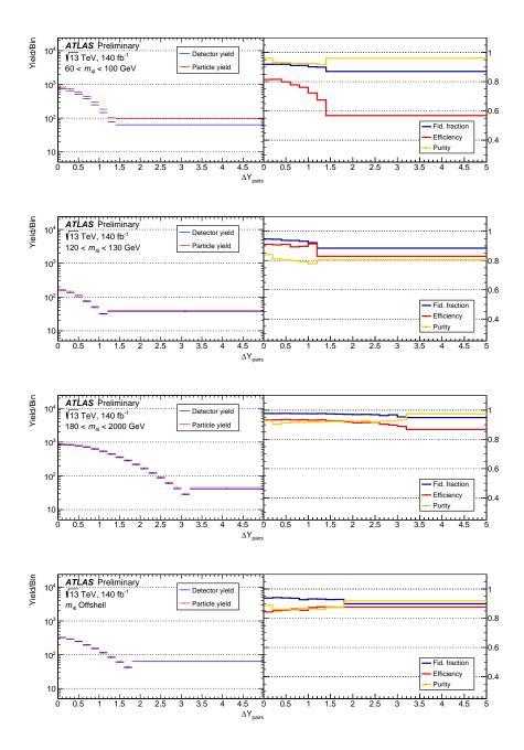
**Figure A.11.:** In the left-hand panels, the number of predicted events passing the reconstructionand fiducial- level selections are displayed as the detector yield and particle yield, respectively. The right-hand panel shows the efficiency, fiducial purity and fiducial fraction. All variables are plotted as a function of the  $|\Delta y_{\text{pairs}}|$  bins, in slices of the  $m_{4\ell}$  variable which are stacked and labelled with the included  $m_{4\ell}$  range.
