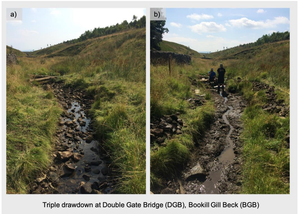
Figure 2.11 Triple Drawdown (TDD) at Double Gate Bridge (DGB), Bookill Gill Beck (BGB), a) before and b) during dewatering.
