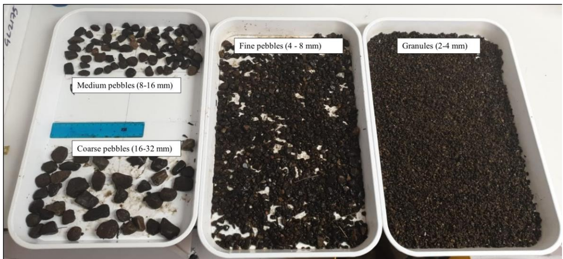
Photograph of substrate in white trays, including; coarse pebbles (13 – 32 mm), medium pebbles (8 – 16 mm), fine pebbles (4 – 8 mm) and granules (2-4 mm).
