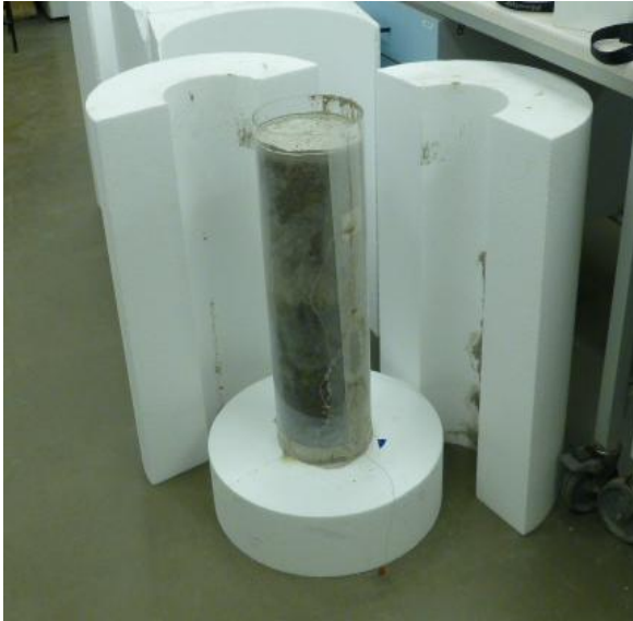
Fig.2: The acrylic cylinder containing concrete with the 200mm encasing insulation removed.
