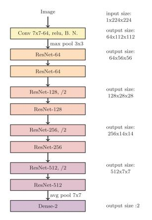
Figure 8. Architecture of the ResNet deep compressor. This network compresses the Kaiser–Squires weak lensing map into a 2D summary statistic, which is constructed to be informative with respect to our two unknown cosmological parameters. These informative summaries are evaluated for all the many simulated mock data maps and the single observed data maps to be used for the likelihood-free inference step.
