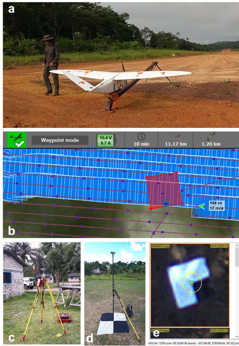
Figure 2. (a) The UAV prepared for launch in Gabon, using conventional take-off and landing (CTOL) procedure aided by a catapult. (b) An example mission over the same study area with flight lines and an approximate image footprint. (c) A static GNSS receiver, the data from which is used to correct the flight trajectories, with additional refinements and corrections possible via ground control points (d + e), located across the study area, the location of which are measured using a “rover” GNSS receiver.
