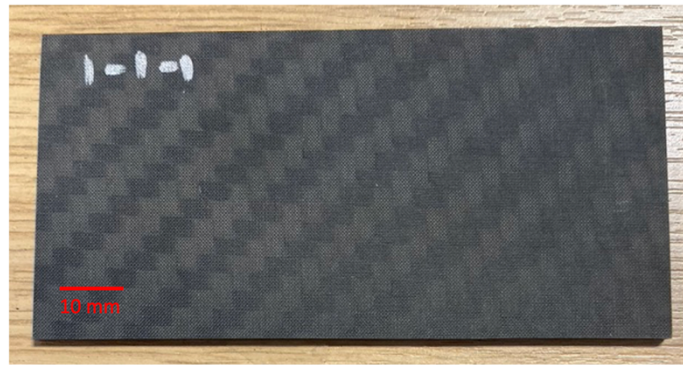
Figure 6-2 Specimen 1_1_1 (0.7% porosity); 10 plies woven composite plate, 100x500mm.
