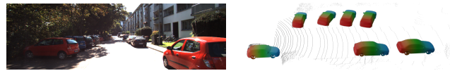
Figure 3: Qualitative shape and pose results on a stereo+LiDAR KITTI sequence. A very sparse set of LiDAR points was used to reconstruct each car. LiDAR points on the road are only shown for illustration.
