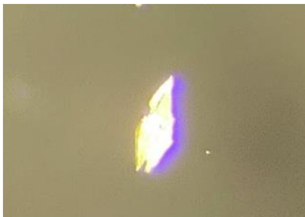
Figure 6.13. Damaged crystals of 6 after incubation in the presence of neat S-nicotine at 25 °C for 1 week. Crystals displayed under polarised light.
