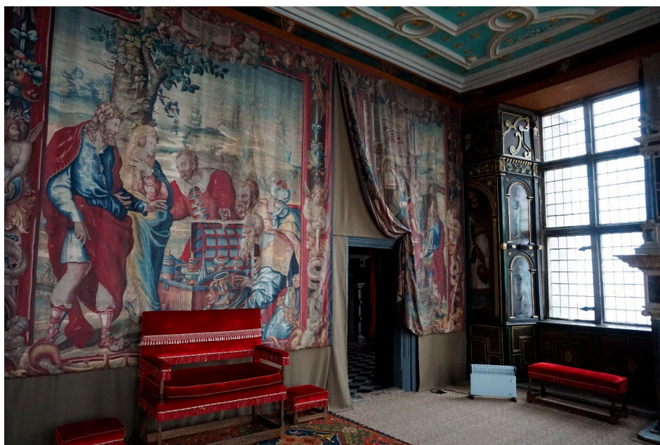
Figure 2. Bolsover Little Castle in Derbyshire, England, which dates from the beginning of 17th century, uses every one of the Stuart period options for providing comfort if one was extremely wealthy. In the Star Chamber, rush mats cover the floor, the walls are hung with cloths and tapestries that also block drafts through doorways, and the windows have both secondary glazing and shutters. Other rooms are similar, or paneled in timber. ©Historic England.
