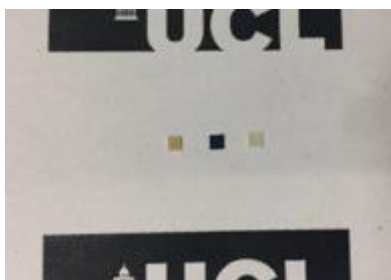
Figure 3.8 Samples of 2 mm x 2mm blank alumina sensor (left), as-deposited WO_3 on alumina sensor(mid) and WO_3 AA on alumina sensor(right)
