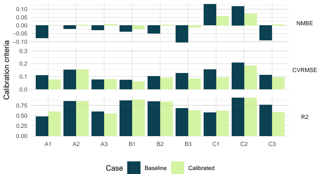
Figure 7.6: Uncertainty criteria for the baseline and calibrated models for each studied archetype (Room B1)
