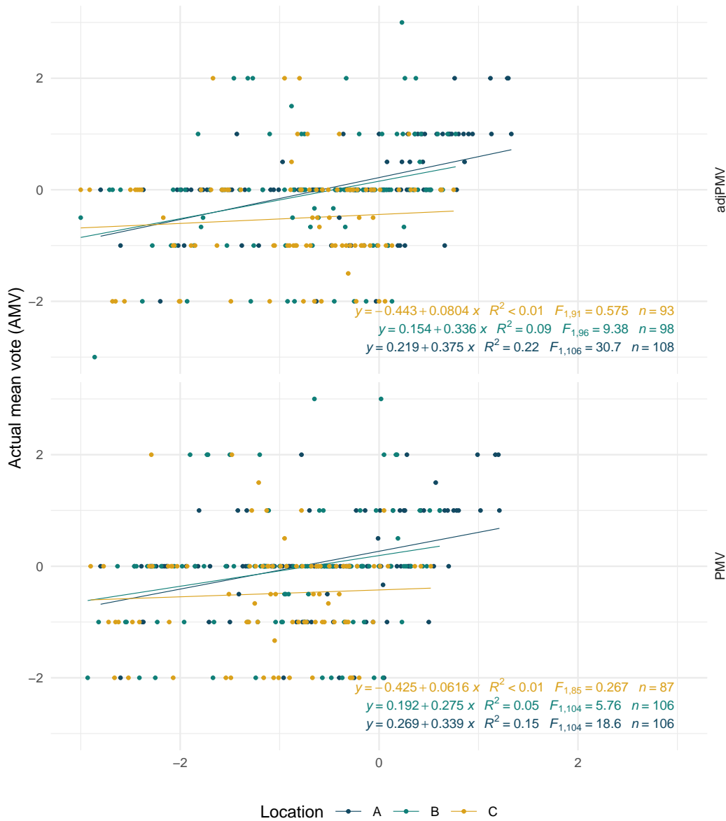
Figure 6.1: Regression of thermal sensation vote (TSV) on the adjusted predicted mean vote (adjPMV)
