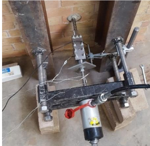
Figure 5-5 Laboratory set up for pull-out test of D-GAS
