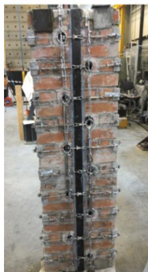
Figure 2-9 Strap/strip technique developed by (Ferretti 2020)
