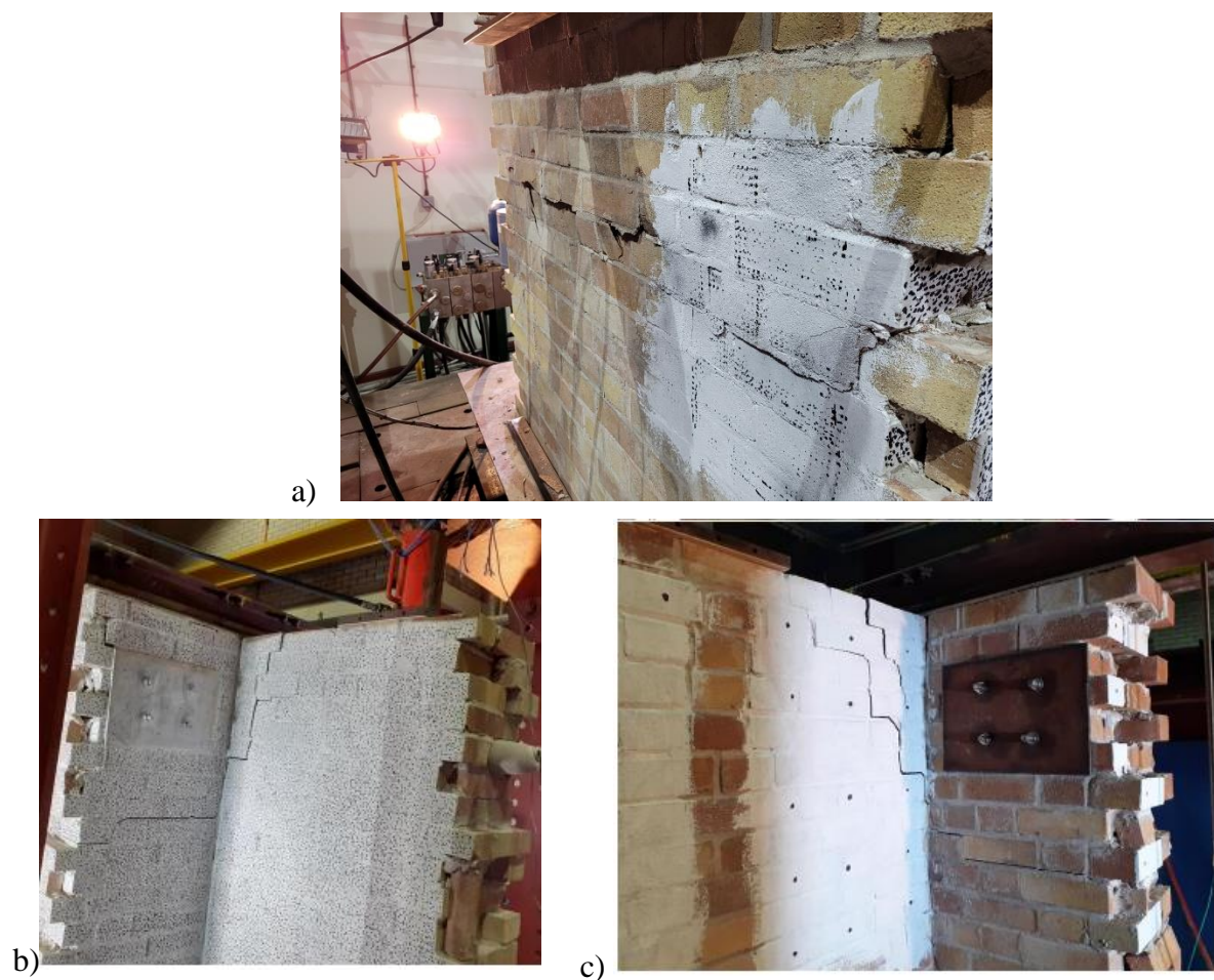
Figure 5-41 Horizontal hinge line and crack propagation on front and spine panels.
