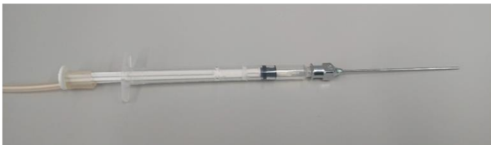
Figure 2.4: Experimental setup for k_{La} measurements in the micro-Matrix (A). A needle-type microsensors (B) was inserted into the well through the off-gas filter and stabilised using a stand. The hood of the micro-Matrix was partially closed to help maintain a temperature of 37°C inside the wells.
