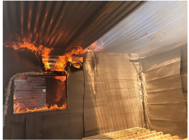
Fig. 11 b) Early spread of flames across the cardboard surface and the polycarbonate sheets starting to melt
