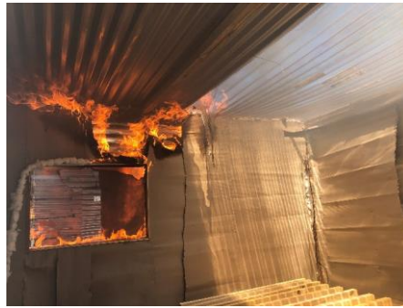
Fig. 11 b) Early spread of flames across the cardboard surface and the polycarbonate sheets starting to melt
