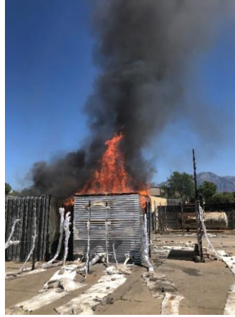
Fig. 23 b) Flames through roof vent of Exp. 3
