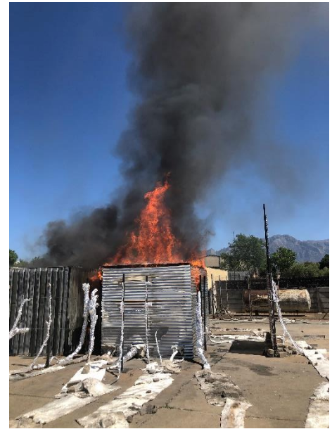
Fig. 23 b) Flames through roof vent of Exp. 3
