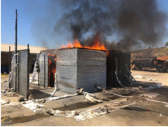
Fig. 23 a) Reduction in flame length emerging out of door for Exp. 3
