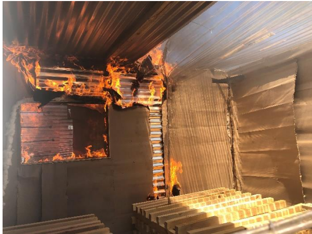
Fig. 11 c) Visual illustration of the melting of the polycarbonate sheets
