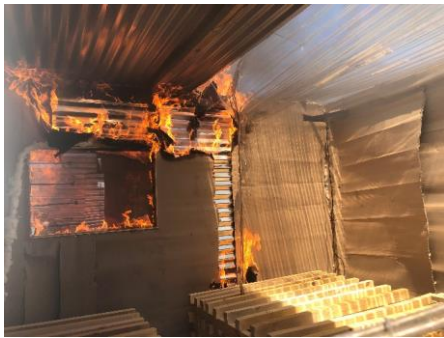
Fig. 11 c) Visual illustration of the melting of the polycarbonate sheets
