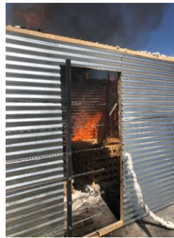
Fig. 11 d) Polycarbonate sheets almost completely melted away
