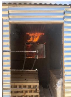
Fig. 10 b) Ignition of the cardboard lining in ISD2 for Exp 2
