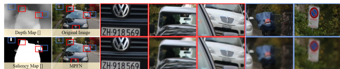
Fig. 19. Some failure results. The red boxes indicate similar saliency regions at different depths, and the blue boxes indicate defocus areas at corresponding depths.
