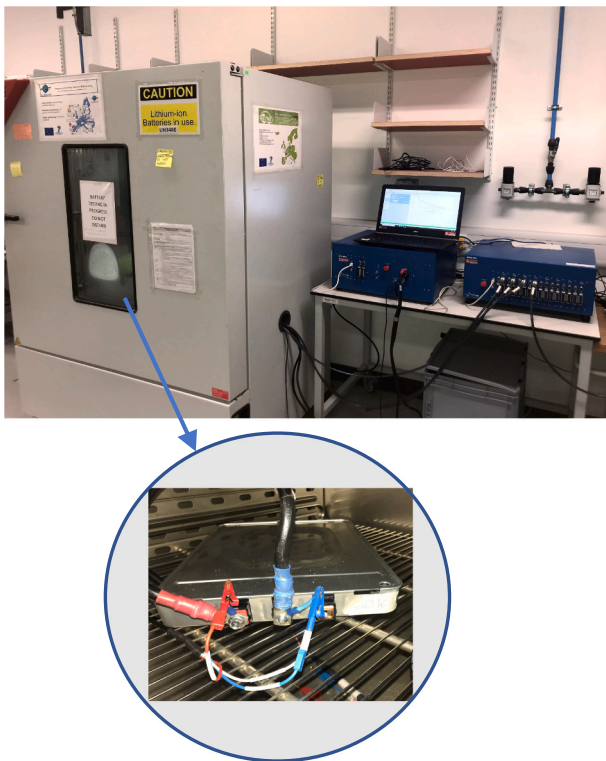
Fig. 5. Configuration of the module test bench.
