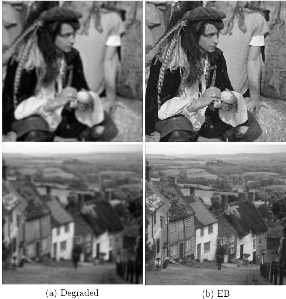
Figure 4.1 – Deblurring with TV prior for man and goldhill test images: (a) blurred and noisy (SNR=30 dB) observation y , (b) MAP estimator obtained using \bar{\theta}_N computed with empirical Bayes.
