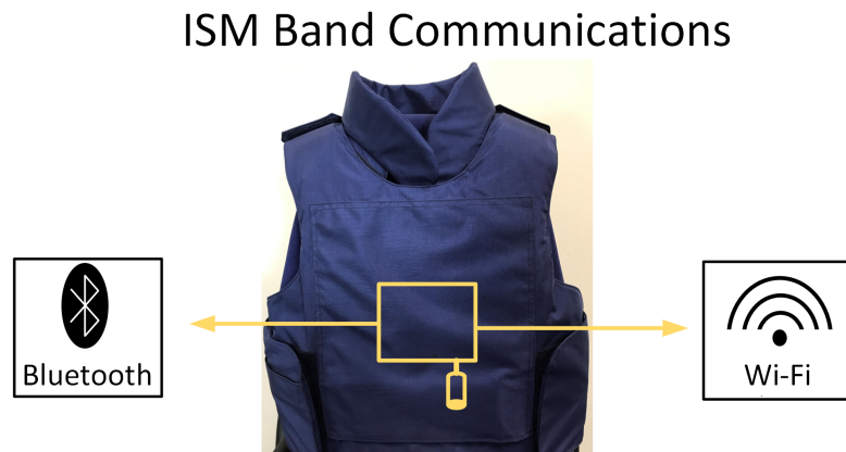
Figure 3.1: Illustration of a wearable antenna intergrated within the ballistics jacket [12].
