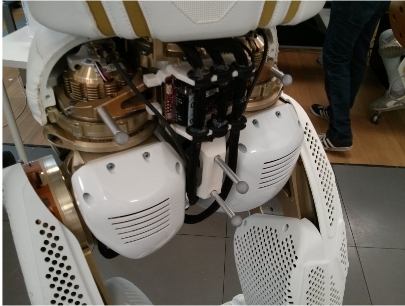
Figure 3.6: Vicon markers are placed on the pelvis to track the pose of the robot during walking.
