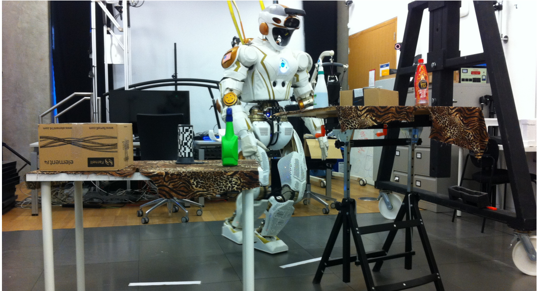
Figure 3.5: The NASA Valkyrie humanoid robot during operation in a laboratory environment. Note the markers on the ground, which are discussed in Section 3.4.3.
