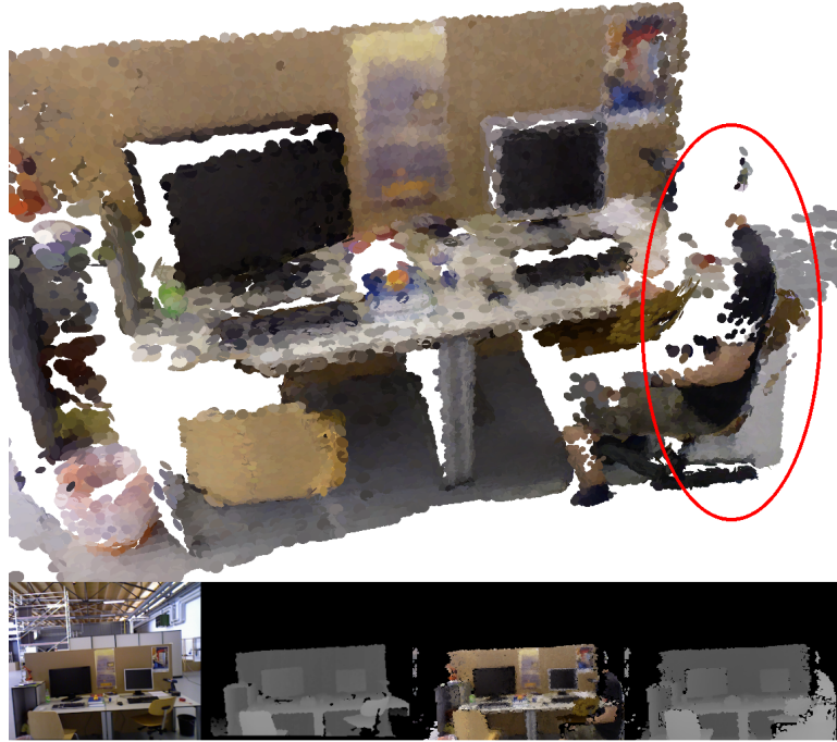
Figure 4.8: Top : An example of a reconstruction which still contains a person even after they have moved (encircled in red). Bottom left : current RGB-D image pair. Bottom right : RGB-D model prediction image pair. The person is not removed from the reconstruction because the current depth image does not contain data in the area where they were sitting.
