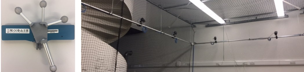
Figure 5.2: Our evaluation set-up. Left: Our Intel RealSense ZR300 camera with mounted motion capture markers. Right: Our Vicon system.
