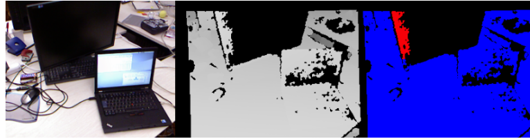
(a) The monitor is incorrectly segmented as dynamic because depth estimation on the black matte monitor is flickery, which results in large residuals.
