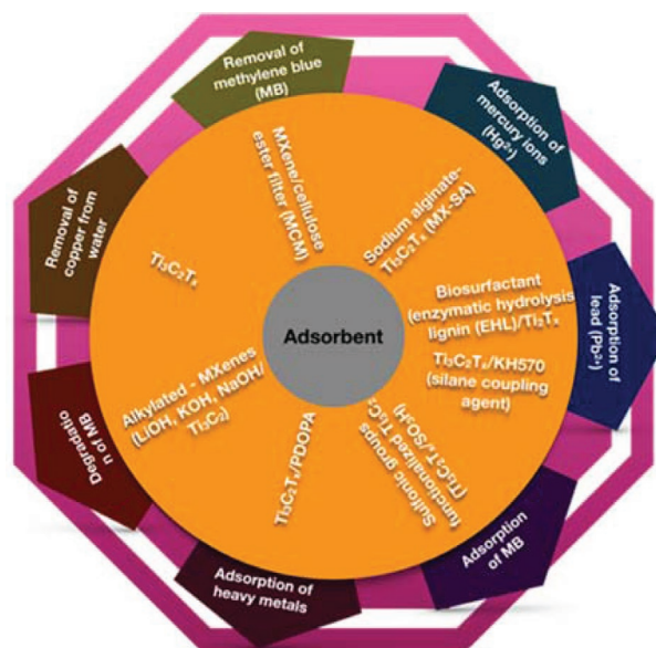
Figure 8. Various applications of surface functionalized MXenes used as adsorbent materials for wastewater treatment.
