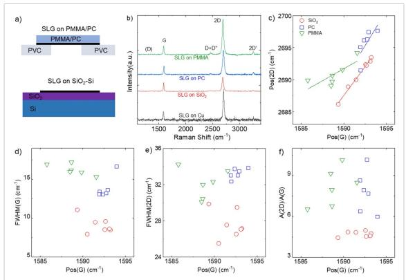
**Figure 1.** (a) Schematic of SLG on PC, PMMA and Si/SiO<sub>2</sub>. (b) Representative Raman spectra of SLG on Cu, SiO<sub>2</sub>, PC, PMMA. (c) Pos(2D) as a function of Pos(G) with linear fitting for each substrate. (d) FWHM(G) as a function of Pos(G). (e) FWHM(2D) as a function of Pos(G). (f) A(2D)/A(G) as a function of Pos(G).
