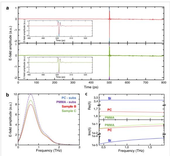
**Figure 3.** (a) Top panel: THz-TDS time traces for (blue) PC bare substrate and (red) SLG on PC (sample B). Bottom panel: THz-TDS time traces measured for (purple) PMMA bare substrate and (green) SLG on PMMA (sample C). (b) Spectra of electric field obtained by Fourier-transforming the time traces in (a). (c) Real (top panel) and imaginary (bottom panel) parts of the refractive indexes of HR-Si (blue curve), PC (red curve) and PMMA (green curve) as from [29, 56].
