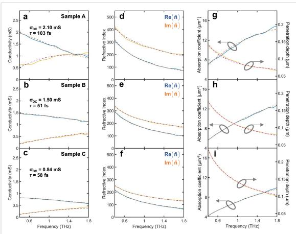
**Figure 4.** (a)–(c) Real (blue) and imaginary (orange) parts of the optical conductivity for samples (a) A (SLG on Si ), (b) B (SLG on PC), (c) C (SLG on PMMA) (from top to bottom). Dashed lines represent the fitting with the Drude model. (d)–(f) Real (blue) and imaginary (orange) parts of the refractive index of samples (d) A, (e) B, (f) C, corresponding to the conductivities in (a)–(c). (g)–(i) Absorption coefficient (blue) and penetration depth (orange) for samples (g) A, (h) B, (i) C.
