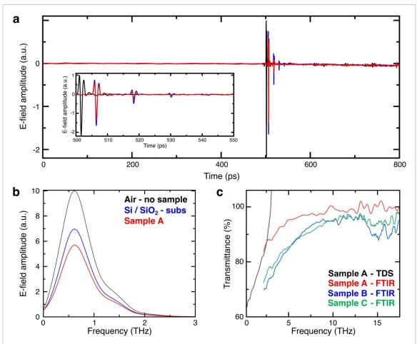
Figure 2. (a) THz-TDS time traces measured without sample (black), with Si reference (blue) and with SLG (red). Inset: zoom of the time traces around the transmitted pulses. (b) Spectra of the electric field associated with the main THz pulse of (a). (c) Comparison between SLG transmittance measured with THz-TDS (black) and with FTIR (red). The FTIR transmittances measured through SLG on PC (sample B) and PMMA (sample C) are in blue and green, respectively.
