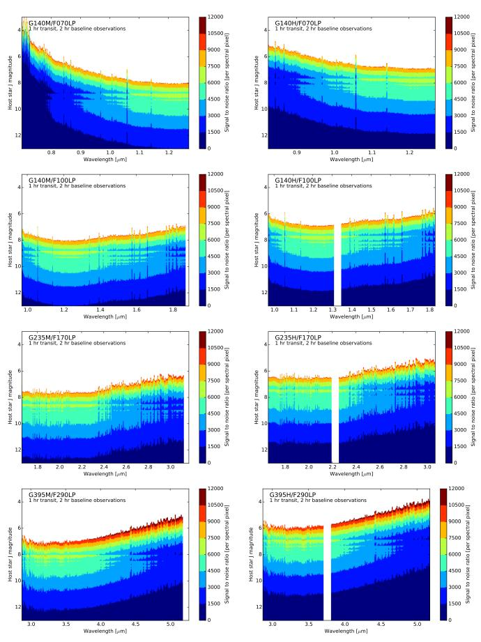
Fig. 6. Signal-to-noise estimates for the high and medium spectral resolution gratings. Based on a host star with effective temperature 3400 K and log(g) = 4.5 (cgs).
