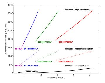
**Fig. 1.** Spectral resolution of the available NIRSpec dispersers. Wavelengths lost due to the small separation between the two detectors in the FPA are represented as a gap in the resolution curves for the high resolution gratings (for the S1600A1 aperture).
