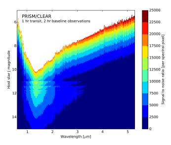
**Fig. 5.** Signal-to-noise estimates for the PRISM configuration based on a host star with effective temperature 3400 K and log(g) = 4.5 (cgs).
