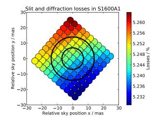
**Fig. 7.** Map of combined slit- and diffraction-losses in the central part of S1600A1 for the grating G235H at 2.45  $\mu$ m. The black circles have radius of 7 and 14 mas, corresponding to 1 and  $2\sigma$  of the allowed pointing drift over 10,000 s, as specified in JWST requirements.
