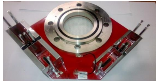
Figure 2: (a) Cranfield University's air-water Serpent Rig experimental facility, (b) Integrated conductance film thickness probe spool with electrolyte injection for film velocity determination, (c) Void fraction capacitance Wire Mesh Sensor (WMS)
