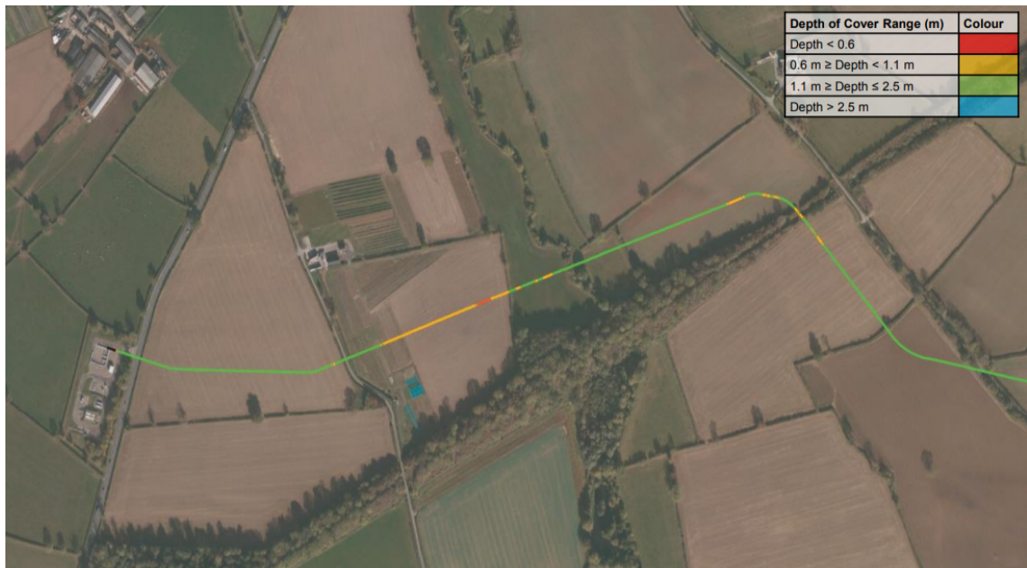
Figure 2.4: Aerial image and example of the results from the depth of cover report. Colours along the pipeline indicate cover depth Published in Finley et al. (2018a).
