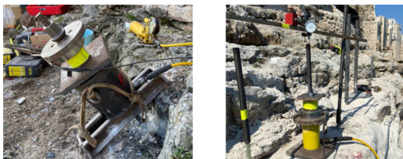
Figure 11. a) Pull test with 1000 kN capacity Hallow piston; b) pull test with 300 kN capacity hallow piston.
