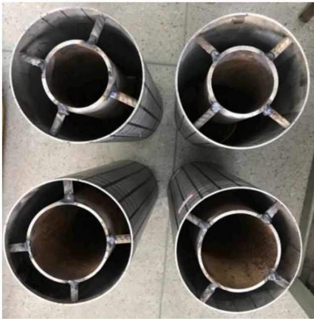
Fig. 1. CFST test specimens before casting.
