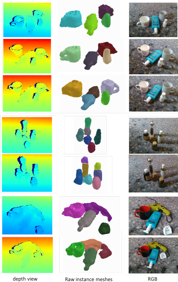
Figure 21: Qualitative results on real scenes with non-convex objects. The raw mesh segmentation of SIMstack is able to estimate shape and decomposition of scenes with non-convex objects.
