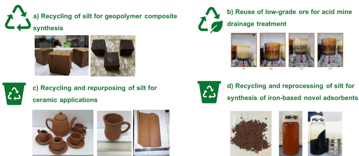
Figure 3: Multi-R approach to nickel-laterite waste management
