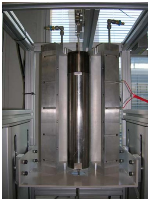
Figure 7.3 View of the pressure vessel, aluminium jacket, thermal insulation box and electrical lift system.
