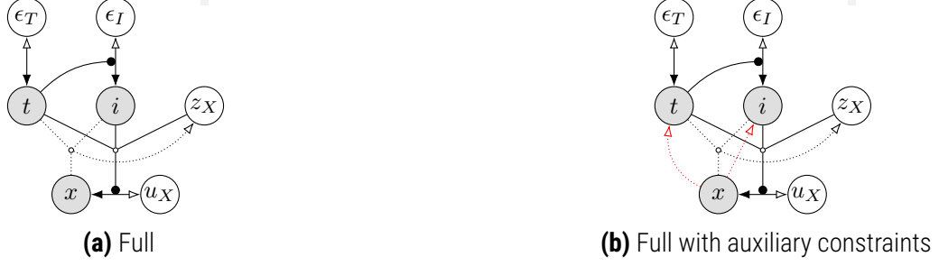
Figure 6.20: Computational graphs of the structural causal models for the Morpho-MNIST experiment studying the effect of correlation in parent variables. The image is denoted by x , stroke thickness by t , and image intensity by i . The corresponding causal diagrams are displayed in the top-right corners. The red dotted arrows from x to i and t in Fig. 6.20b refer to the auxiliary distributions described in Section 6.2.5.
