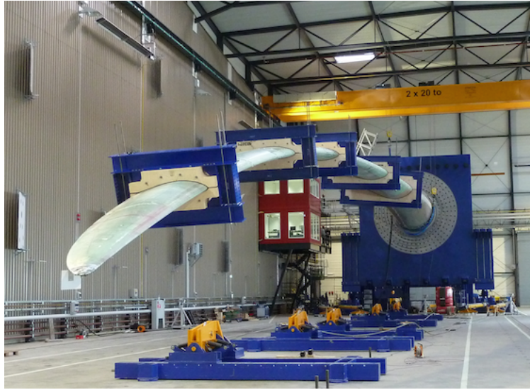
Figure 1.7: Wind turbine blade test. Image from Renewable Energy World https://www.renewableenergyworld.com/storage/substructure-testing-paving-the-way-to-longer-blades/ . Accessed October 5 th , 2021.
