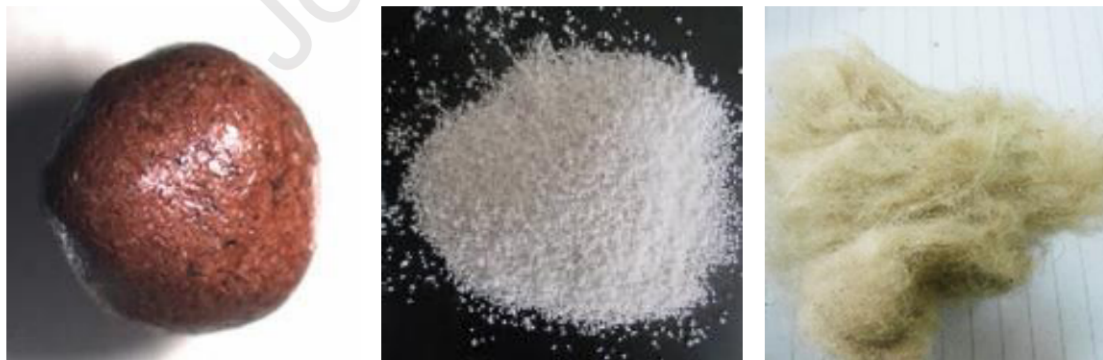
Fig. 5. ( left ) Expanded Clay (EC) particle with styrene-acrylic protective layer [87]; ( middle ) Expanded Perlite (EP) particles [80]; and ( right ) flax porous fibre [122].
