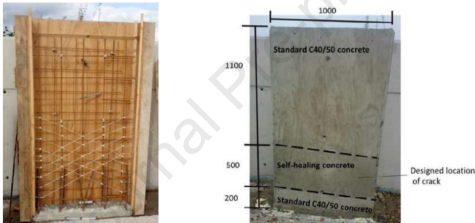
Fig. 9. Bacteria-based self-healing concrete (BBSHC) field trial in the UK: ( left ) vascular flow network installed prior to casting of the BBSHC concrete; and ( right ) vertical wall containing BBSHC (middle zone) and standard C40/50 concrete (dimensions in mm) [153,155].
