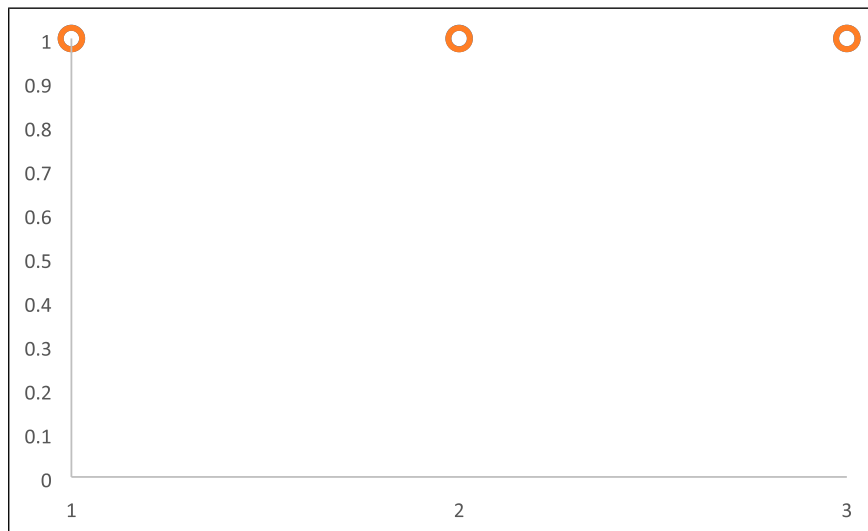
Figure 11. The deviation of first three mode shapes by applying Mode Shape Correlation Coefficient index, blade at rotating speed=12.1 RPM, blade at rotating speed =0 RPM comparing with rotational speed =15 RPM
