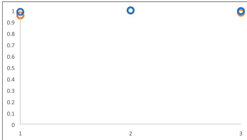
Figure 10. The deviation of first three mode shapes by applying Modal Scale Factor index, blade at rotating speed=12.1 RPM, blade at rotating speed =0 RPM comparing with rotational speed =15 RPM
