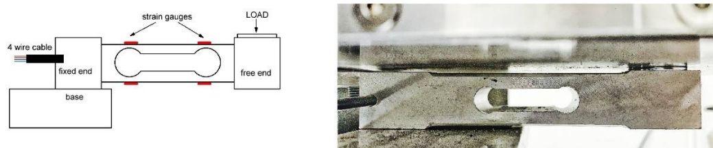
Figure 1. A load cell representation (left) and the load cell used in our device (right).
